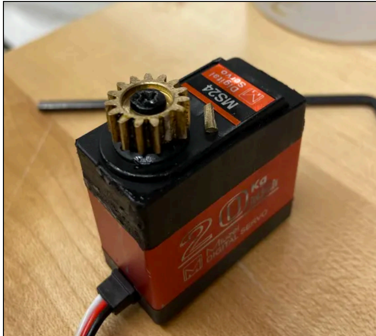
Figure 21: Pinion Gear with Sheared Tooth Following Impact Testing
