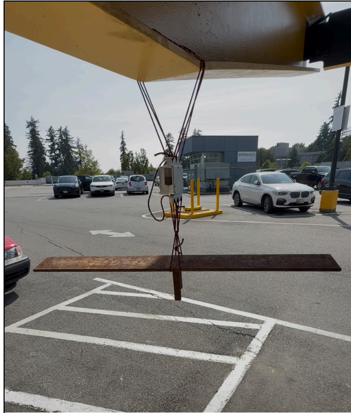
Figure 17: Drop-off Tensile Stress Testing Setup
